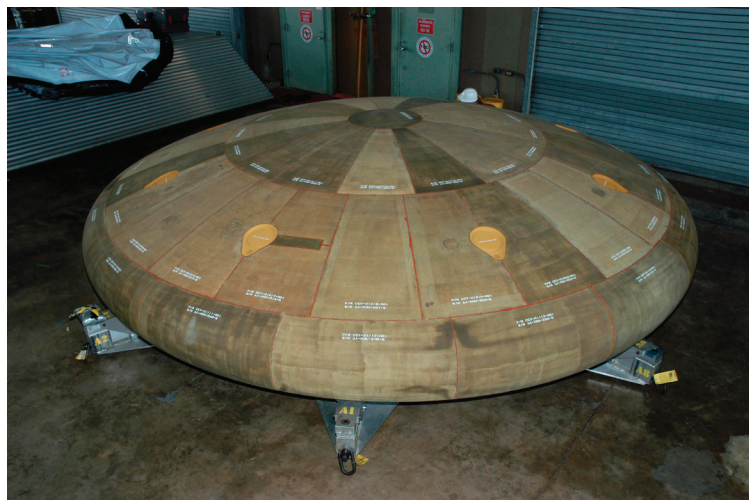
A developmental heat shield for the Constellation crew exploration vehicle, or CEV, is being prepared for a demonstration at NASA's Kennedy Space Center.
