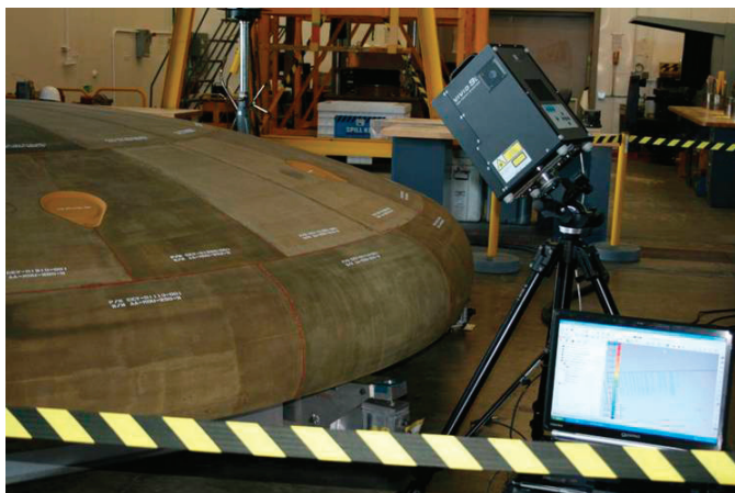
A laser scanner system at Kennedy is being used to obtain a surface profile of the MDU.
