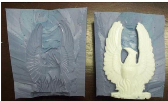
Figure 3 – RTV silicone mold and urethane casting
