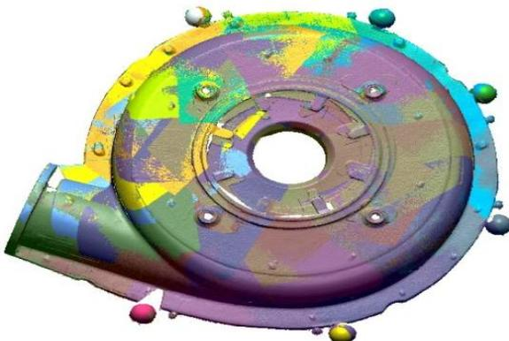
Figure 2 – Scanned Data Patches
